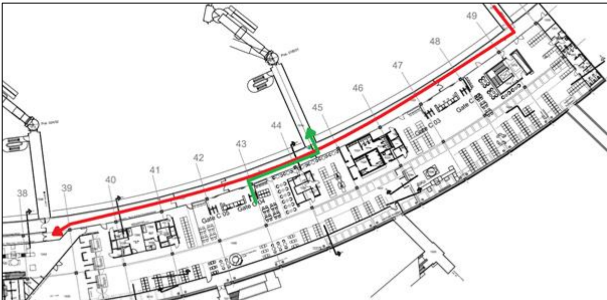
Figure 12: Example of intersecting clean and unclean passenger flows in northern Passenger Pier Arriving unclean passengers (red arrow) partially use the boarding corridor for departing passengers (green arrow). If boarding of departing passengers has commenced, it must be interrupted; boarding can only commence or resume once Passenger Services have inspected the corridor section used by unclean passengers.
